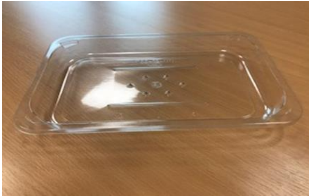
Figure 4: Original PET tray with sealing layer and top film, made with 95% recycled materials.
