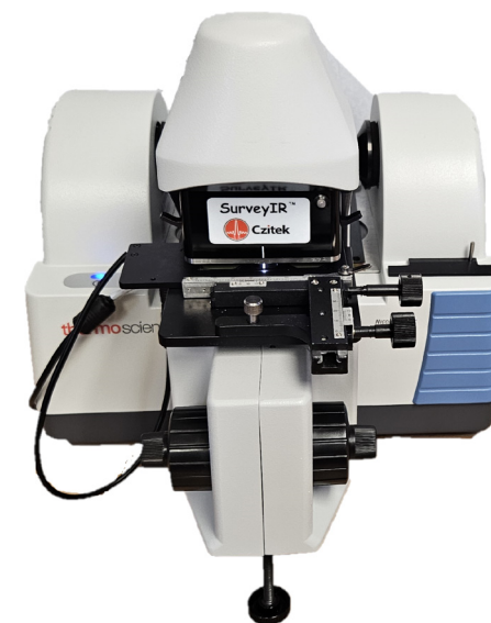
Image of a Nicolet IS5 with a SurveyIR accessory.
