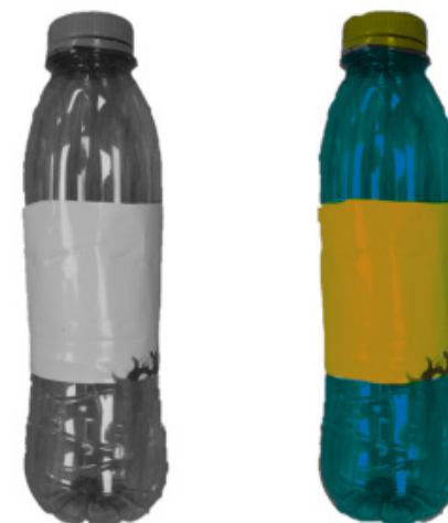
Above: colour map image showing how a PET bottle with a PP label covering 60% of the bottle could be viewed by an NIR operating in a MRF.
