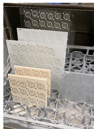
Figure 6. Placement of the compression moulded sheets with the type A tags in the commercial dishwasher.
