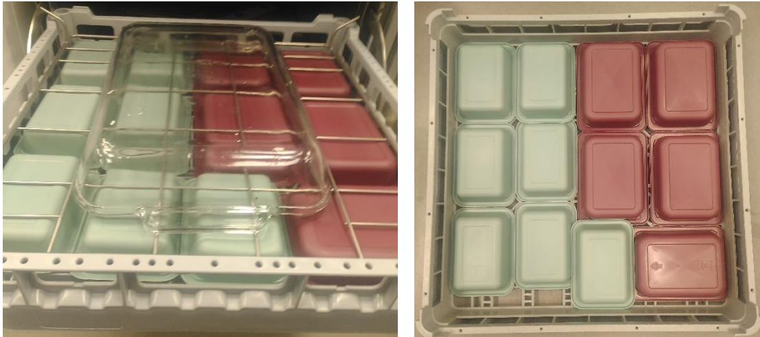
Figure 3. The cPET samples are arranged in the Classeq D500 under-counter washer. The metal grid and Pyrex dish weigh the containers down and prevent them from being flung around the dishwasher. The washing tray is 500mm x 500mm for scale.
