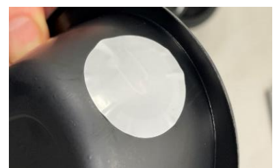
Figure 12. Samples with low radii of curvature in two dimensions showed the expected wrinkling due to the limited flexibility of the tag.
