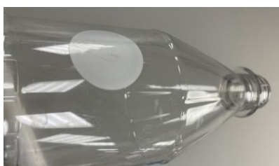
Figure 10. Tags adhered well to containers with curvature in one
