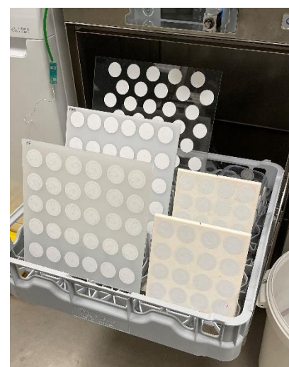
Figure 7. Type B tags on PBT, PP, HDPE and amorphous PET flat sheets. Tags on Tritan sheets were washed separately
