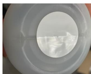
Figure 13. Wrinkling is present when the tag is applied to the base of a bottle
