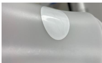
Figure 11. Sample with curvature in two directions. Showing good tag adhesion.
